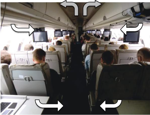
FIGURE 2. Ventilation system and subjects in the Do 728 mock-up © DLR
