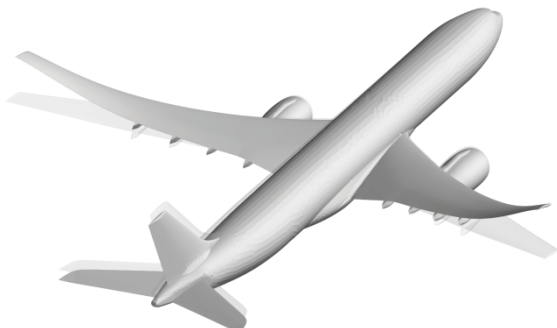
FIG 4. Visualization of the first elastic eigenmode mainly exposing a symmetric bending of the wings.
