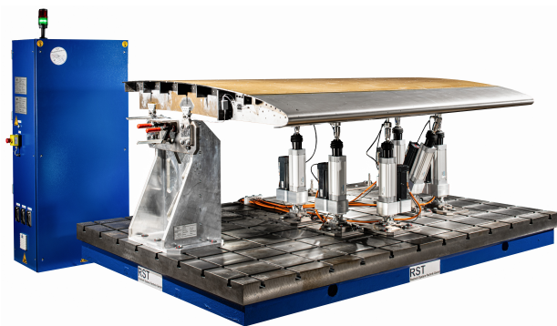
FIG 2. Test rig for mounted leading edge with ground and flight loads
