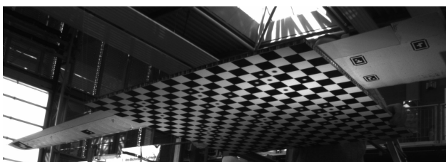
FIG 11. CamS 1 calibration image with checkerboard pattern
