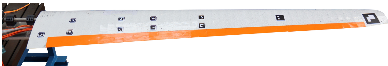
FIG 5. Test rig setup of the AdLoNet prototype wing in laboratory testing as part of calibration tests with CamS markers on the wing surface
