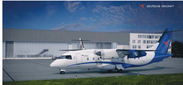
Fig 6: Rendering of the 328-100 based technology demonstrator with additional E-motors developed by GE
