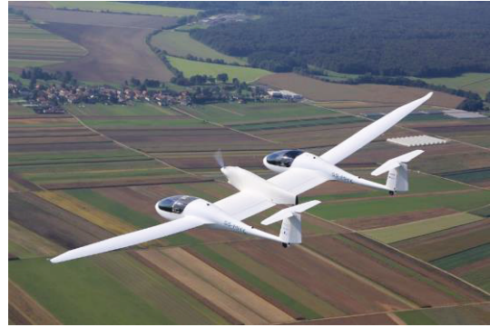
Fig 3: HY4 flying platform with 50 kW fuel cell propulsion system
