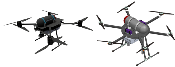
FIG 2. Preliminary UAV design concepts; left: coaxial octocopter [10], right: hexacopter [11]
