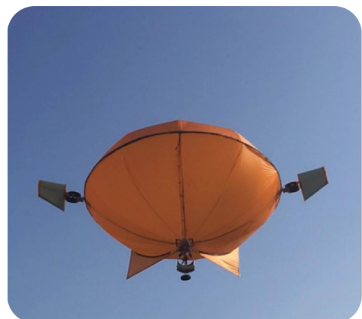
Figure 1 h-aero ® one, 3kg payload, 5h endurance
